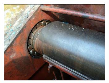
Bearings rusted and in poor condition due to lack of lubrication.
