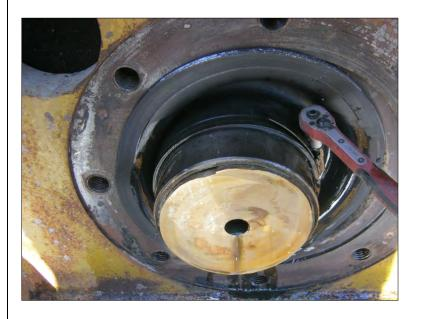
New seal fitted to swing jaw guide.
