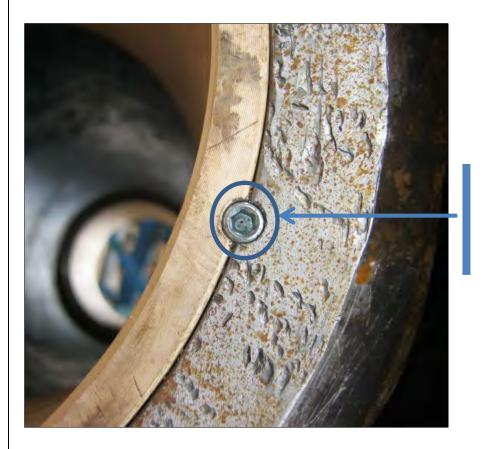
Both Bushes fitted and held with grub screws to ensure bush does not move.
