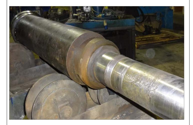
Damaged pitman shaft
