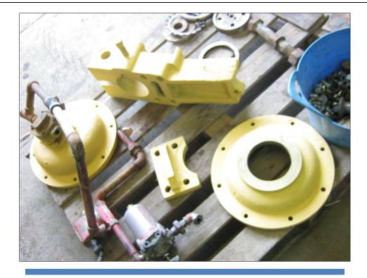
Pump striped and cleaned with new gasket set.
