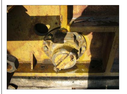
Swing jaw guide striped down for inspection.
