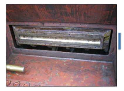
Damaged diaphragm removed and diaphragm frame holes re-tapped.
