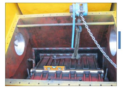
Pitman toggles and toggle pin fitted.
