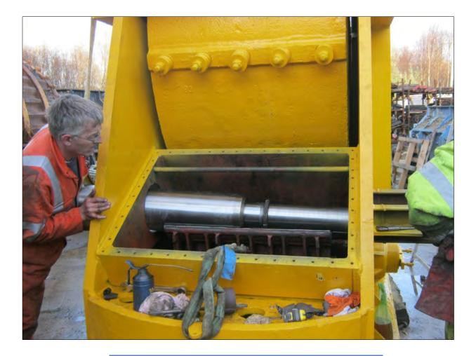
Eccentric shaft and bearing assembly being fitted
