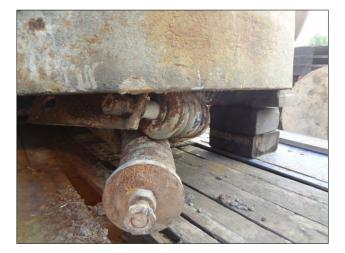
Damaged draw back bolts that we replaced. Sump plate bolts missing, we re-drilled and taped damaged holes and fitted new bolts c/w a new cover plate.
