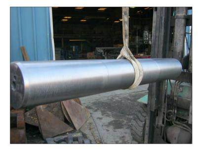
New hinge pin ready to be fitted.
