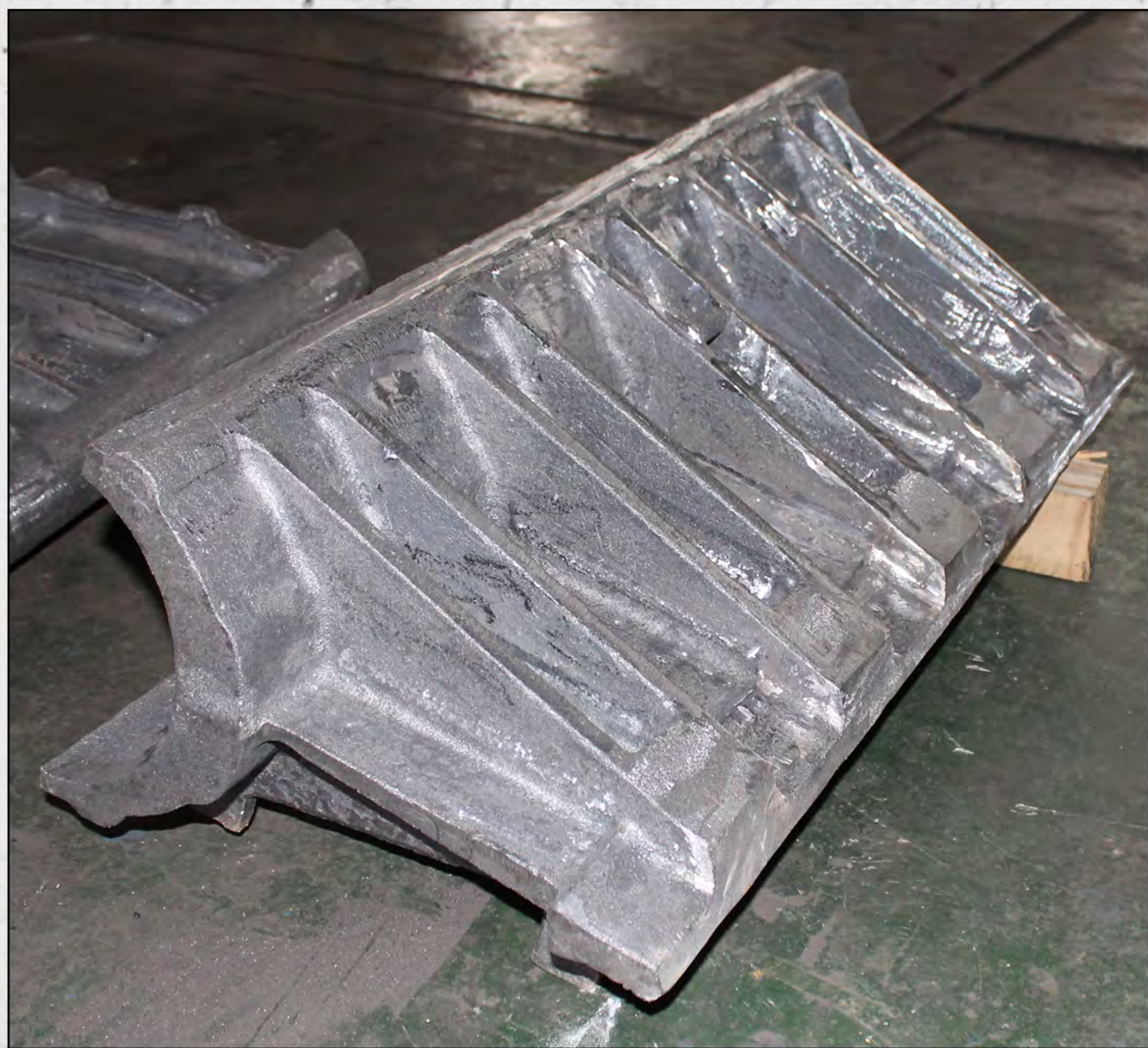
PITMANS & TOGGLE PLATES PRIOR TO MACHINING
