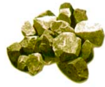
STONE CRUSHED BY A KUBITIZER IMPACT BREAKER
