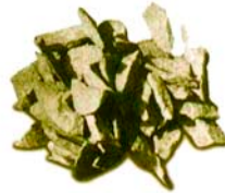
STONE CRUSHED BY A TRADITIONAL JAW CRUSHER
